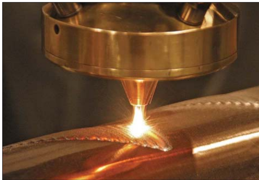
This CO 2 laser is melting the matrix of tungsten carbide powder cladding material and fusing it to an oil field grade stainless steel tubular (Fig. 1; photo by Laser Cladding Services Ltd.).
