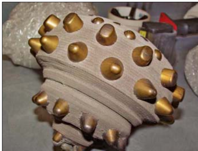
The carbide inserts of this 8-in. OD drillbit were clad with a dissimilar metal to protect the wear surfaces and extend service life (Fig. 4, photo from Laser Cladding Services Ltd.).
